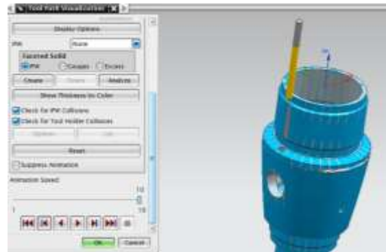
Fig shows Drilling operations and verification DEVELOPMENT OF FIXTURE Below image shows sketch and revolve of fixture
