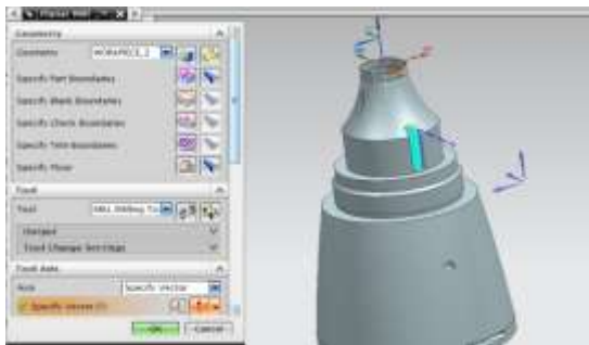
Fig shows planar mill operations and verification Below image shows Drilling operations and verification
