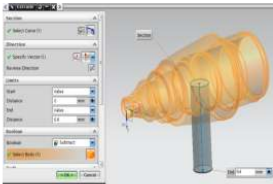
Fig shows sketch and Extrude of Fuze shell
